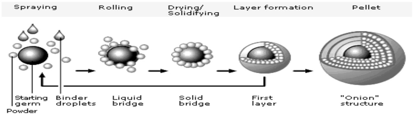
Fig. 2: Principle of powder layering
