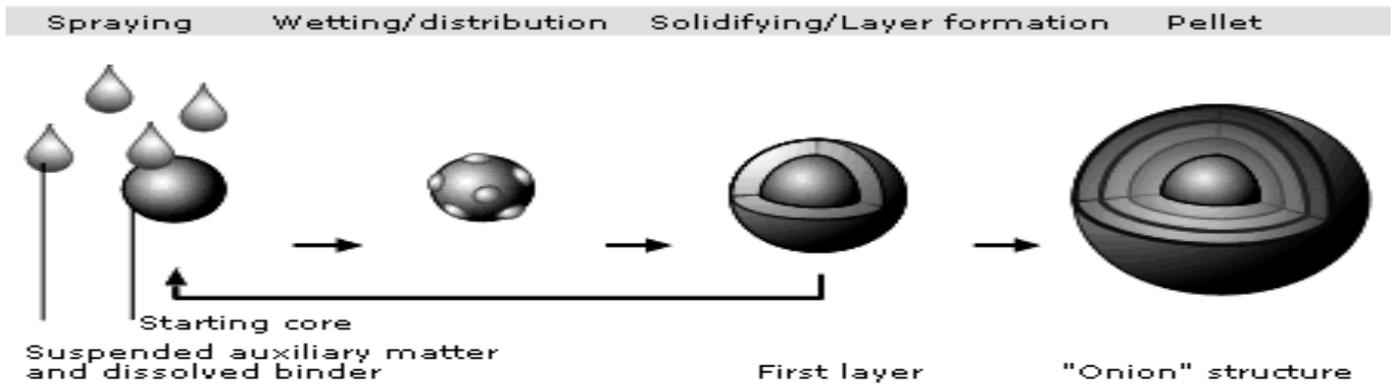
Fig. 1: Principle of solution and suspension layering
