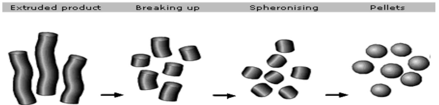
Fig. 3: Principle of spheronization process
