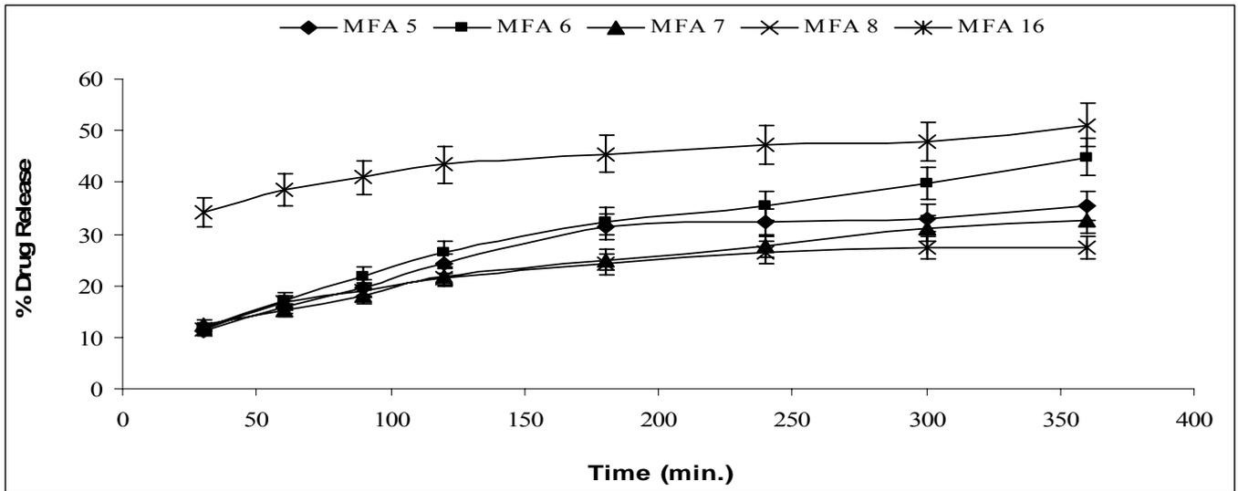
Fig. 5: Dissolution profile of pure Mefenamic acid (MFA-16) and its formulations prepared by solvent evaporation (MFA-5 – MFA-8)
