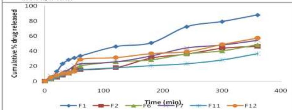
Fig. 4: Comparison of dissolution profiles of metronidazole tablets formulated with binders at 2%, 4% and 6% w/w conc.
