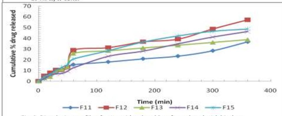
Fig. 3: Dissolution profile of metronidazole tablets formulated with binders at 6% w/w conc.
