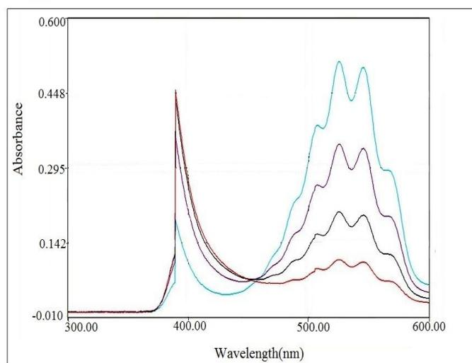
**Fig. 5:** Spectral changes during the oxidation of ciprofloxacin (CIP) by permanganate in acidic medium at 25°C: [MnO<sub>4</sub><sup>-</sup>] =  $2.0 \times 10^{-4}$ , [CIP] =  $2.0 \times 10^{-3}$ , [H<sup>+</sup>] =  $1.0 \times 10^{-2}$  and  $I = 0.05/\text{mol dm}^{-3}$ .
