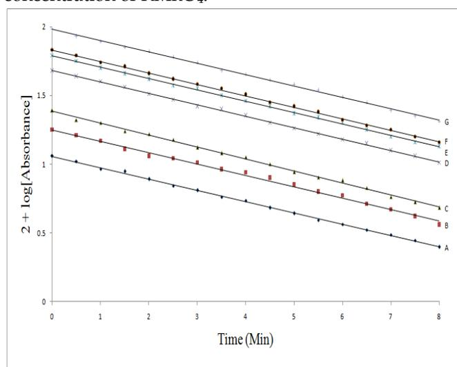
Fig. 3: First order plots of the variation of permanganate concentration at 25°C.  $[\text{CIP}] = 3.0 \times 10^{-3}$ ,  $[\text{H}^+] = 1.0 \times 10^{-2}$ ,  $I = 0.05/\text{mol dm}^{-3}$ ,  $[\text{MnO}_4^-] \times 10^{-4} \text{ mol dm}^{-3} =$  (A) 0.75, (B) 0.50, (C) 1.0, (D) 2.0, (E) 2.5, (F) 3.0, (G) 4.0.
