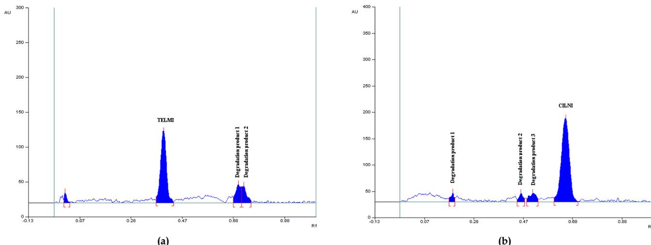
Fig. 5: Representative densitogram after oxidative degradation (a) TELMI with degradation products at Rf 0.70, 0.74 (b) CILNI with degradation products at Rf 0.20, 0.45, 0.50
