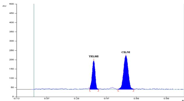
Fig. 1: Representative densitogram of mixed standard solution of TELMI (600 ng band<sup>-1</sup>, R<sub>f</sub> = 0.38 ± 0.03) and CILNI (300 ng band<sup>-1</sup>, R<sub>f</sub> = 0.62 ± 0.05)
